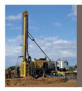
Mining drilling is the process of drilling a hole in the ground for the extraction of a natural resource gold, copper, iron and nickel, for the injection of a fluid from surface to a subsurface reservoir or for subsurface formations evaluation or monitoring. Drilling for the exploration of the nature of the material underground (for instance in search of metallic ore) is best described as borehole drilling, or 'drilling'.
