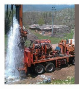
Water Well Drilling is the process of drilling a hole in the ground for the extraction of underground water, for the injection of a fluid from surface to a subsurface reservoir or for subsurface formations evaluation or monitoring. It is a fast way to find water.
