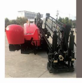
Horizontal Directional Drilling is a steerable trenchless method of installing underground pipes, conduits and cables in a shallow arc along a prescribed bore path by using a surface-launched drilling rig, with minimal impact on the surrounding area. Directional boring is used when trenching or excavating is not practical. It is suitable for a variety of soil conditions and jobs including road, landscape and river crossings.
